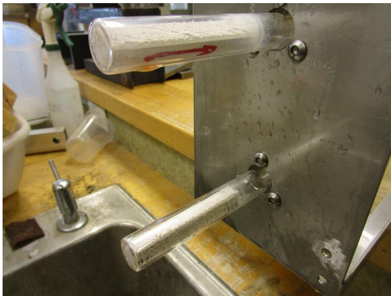
Photo No. 4 ASTM E228 - CLTE - Specimen Detail
