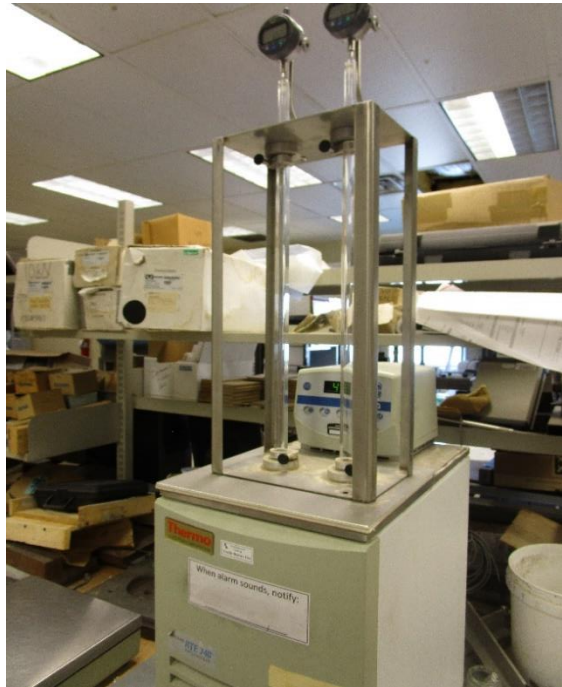
Photo No. 3 ASTM E228 - CLTE - Equipment Detail
