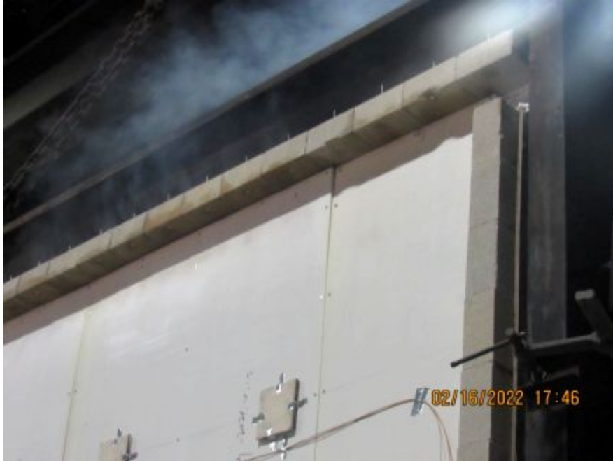
Photo No. 11 Wall popping out at joint
