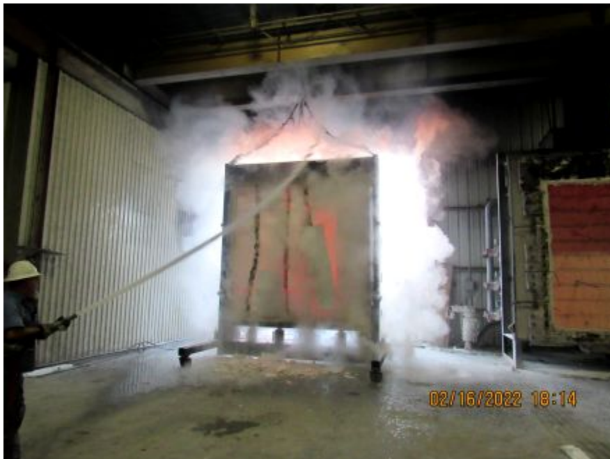
Photo No. 16 Start of Hose stream test
