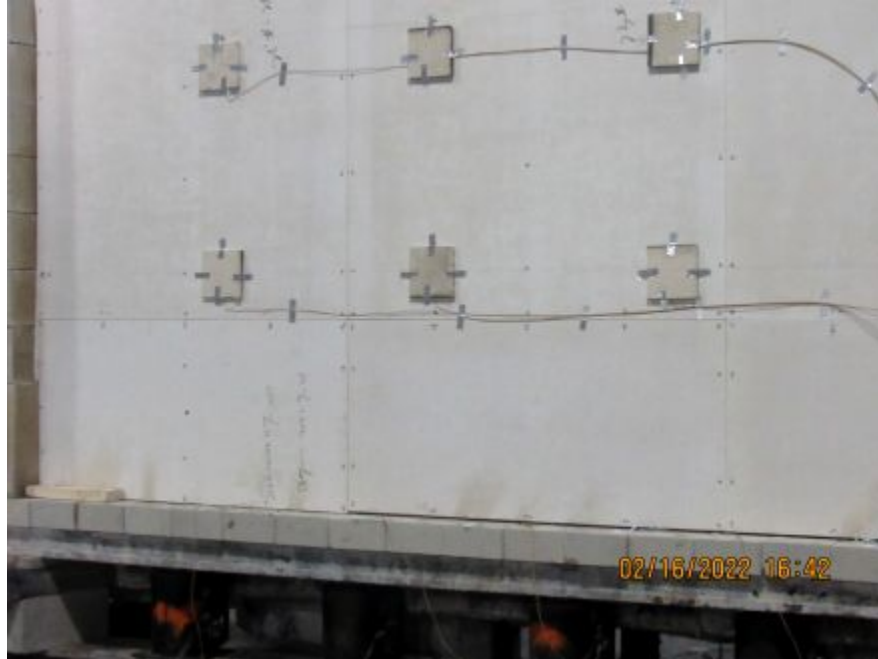
Photo No. 9 Discoloration on bottom of boards
