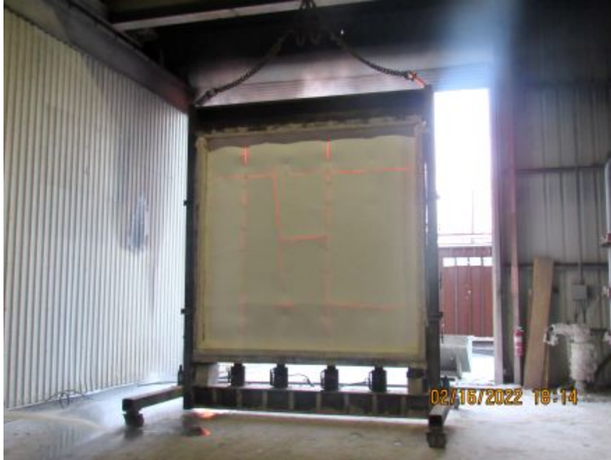
Photo No. 15 Exposed side post-fire exposure
