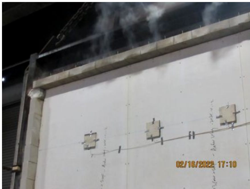
Photo No. 10 Discoloration on joints
